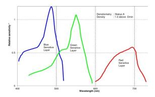
\*Sensitivity equals the reciprocal of the exposure (j/cm²) requires to produce a specified density
